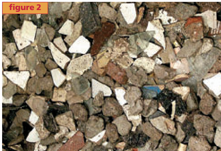
Figure 1 Light fraction of 20-40 mm from mixed C&D waste at the plant of Van Gansewinkel in Vlaardingen, The Netherlands, where the samples were collected.
