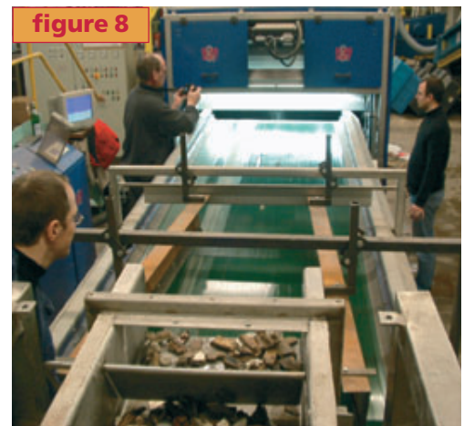
Scan & Sort CombiSense at the Technical University of Aachen in Germany
