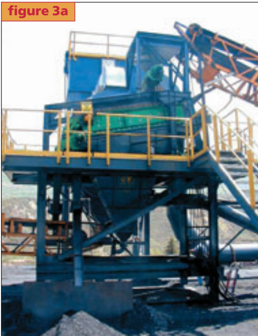
A 50 tonnes per hour air jig used for cleaning coal. (Photo: Allmineral/Technical University of Aachen, Germany)
