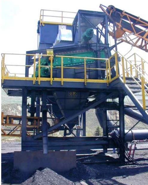
Fig. 3a – 50 t/h air jig for the cleaning of coal (Allmineral, RWTH Aachen).
