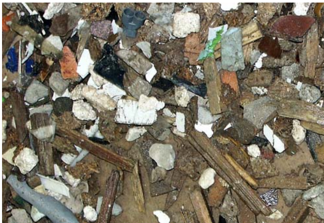
Fig. 1 – 20-40 mm light fraction from mixed CDW at the Vlaardingen plant of Van Gansewinkel, The Netherlands, where the samples were collected.
